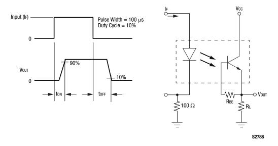
Figure 6. OLS100 Switching Test Circuit
