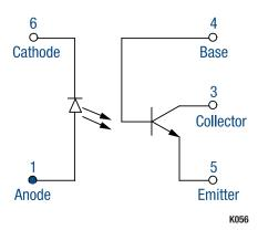
Figure 1. OLS100 Block Diagram
