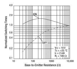
Figure 5. Normalized Switching Times vs Base-to-Emitter Resistance
