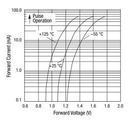
Figure 2. Forward Current vs Forward Voltage
