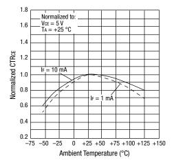
Figure 4. Normalized CTRcE vs Temperature
